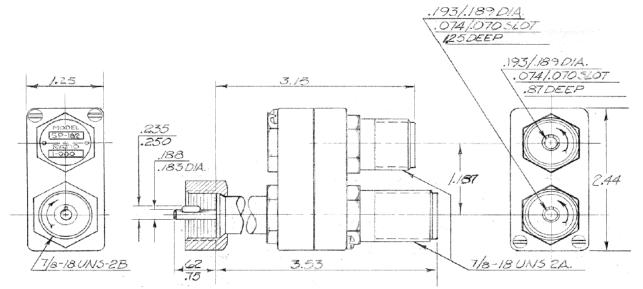
The Splitter Drive is shown below with an RA Adapter added to one of the output ports. The second port will normally connect to a drive cable or a different adapter for a secondary output.
