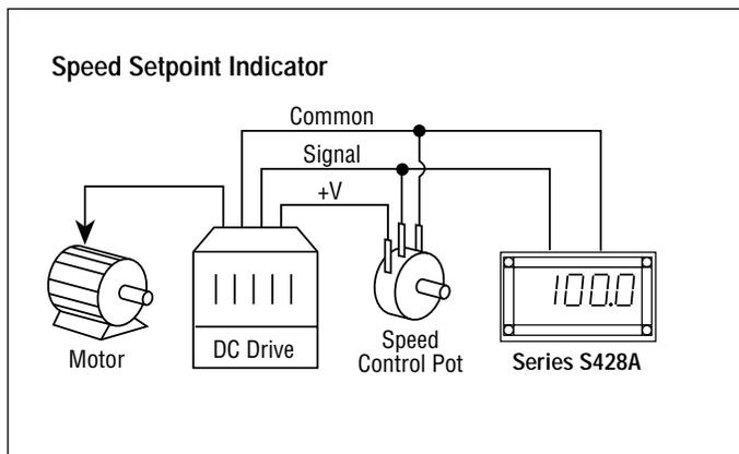
**DC Current Meters** are popular when noise interference can disrupt voltage levels and are common signals used to drive old analog meters. Reference outputs of 0 to 1 mA, 0 to 5 mA, and 0 to 10 mA which are proportional to motor speed are also available from some AC drives.
