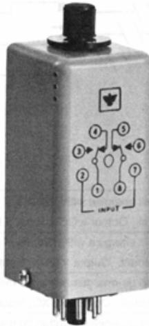
The CG900 series is a delay timer available in 19 time ranges from 0.5 seconds to 30 hours. The timer uses CMOS integrated circuits for the timing function. The desired delay time is set by the adjustment of a calibrated knob referenced to an index mark on the housing. At time out, a DPDT relay is actuated for control of output loads.
