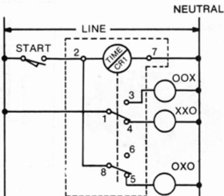
NOTE: Schematic diagram is for typical application with 120 VAC supplying both control input and load power. When control input and load voltages differ, this diagram must be modified to separate the two voltage sources.
