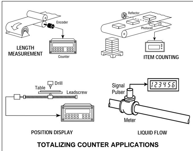
Today's electronic totalizers bring the advantages of modern digital displays, high counting speeds, silent operation and long life. Our general purpose types are comparably priced to other technologies and are very easy to install and use. Their high speed and compatibility with a variety of sensors makes them ideal for precise measurement of length or position, as well as totalization of fast moving items, liquid/gas volume, and other demanding tasks.
