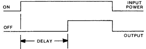
ON DELAY: Time delay starts upon application of power. Relay energizes after delay. De-energizing input terminals resets timer.
