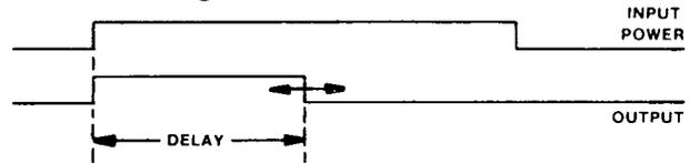
Interval: Upon application of power, timing begins and output relay is energized. Output relay de-energizes at time-out. Removal of input power resets timer.
