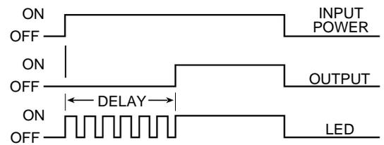
ON DELAY: Time delay starts upon application of power. Relay energizes after delay. De-energizing input terminals resets timer.
