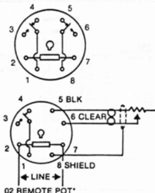
The wires from the remote potentiometer must be a shielded twisted pair connected to terminals 5 and 6 the octal socket. The shield must be connected to terminal 8. The shield must remain unconnected (floating) at the potentiometer end of the cable. Cable length cannot exceed 12 feet.
