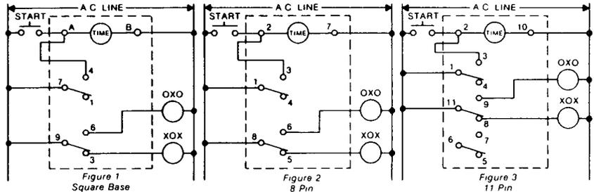
**ONE SHOT** — Momentary or Maintained start switch. Close switch to start timing. Resets automatically using momentary start. Resets upon opening maintained switch. Relay contacts provide interval sequence (OXO, XOX). Contacts 4-7 (E and H Series) must be wired as shown for one shot control (Figure 1). For Q Series wire contacts 3-1 as shown in Figures 2 and 3.
