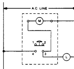
By placing a jumper between terminals 1 and 4 of switch, a form "C" SPDT switch is obtained. When manually depressed, push-button switch is mechanically latched in the "4-3" closed position. At time out, latch is released and "4-3" opens.
